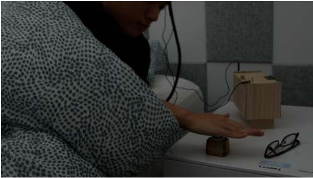
Figure 4: Our system includes an emergency stop feature in the event the user is uncomfortable or distressed to cease the ongoing stimuli.
